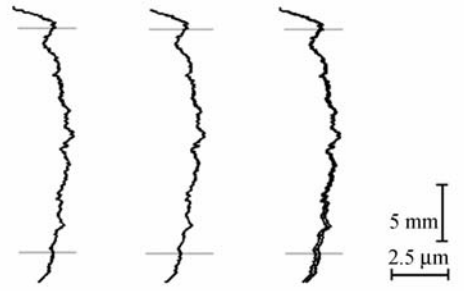
(a) 齿根至齿顶 (b) 齿顶至齿根 (c) 重合放置 (a) From root to tip (b) From tip to root (c) Overlapping
